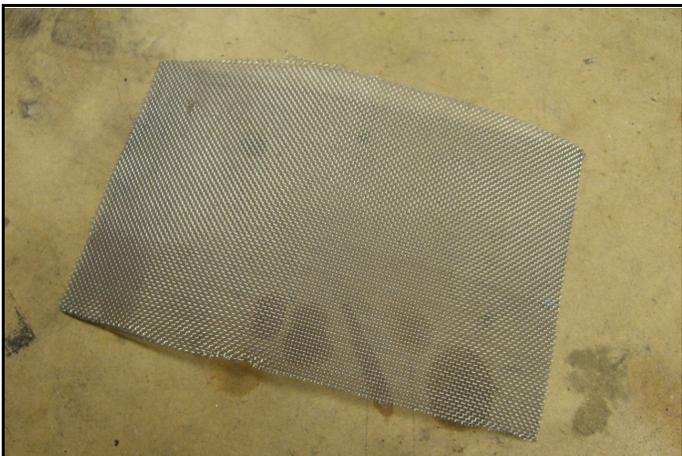
Cut a length of fine stainless or aluminium wire mesh
