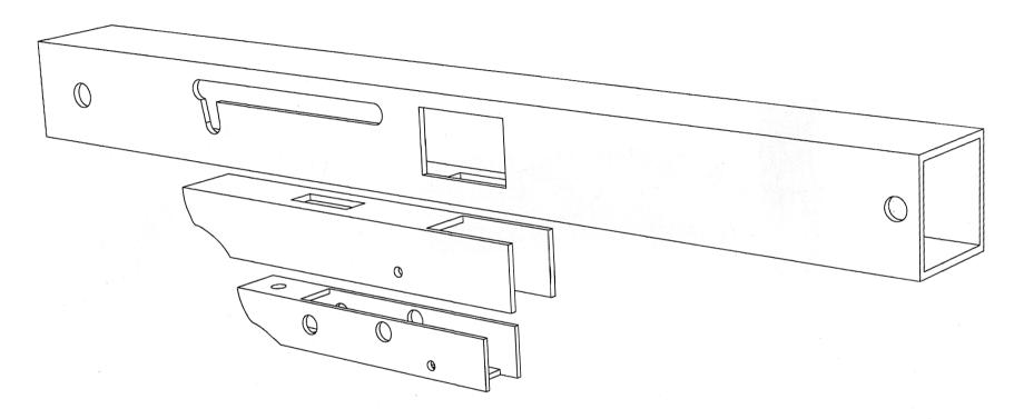
THE UPPER, LOWER, AND TRIGGER GROUP RECEIVERS SHOWN IN THEIR CORRECT ASSEMBLY POSITIONS
