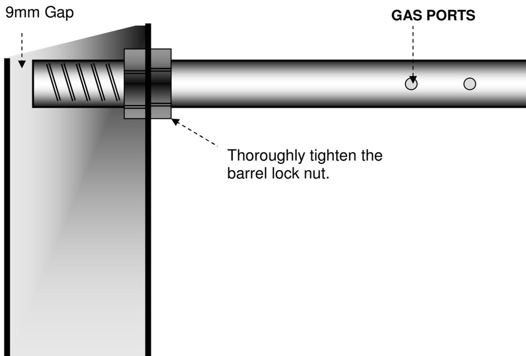
*With the barrel fitted we can proceed and fit the striker assembly.*
