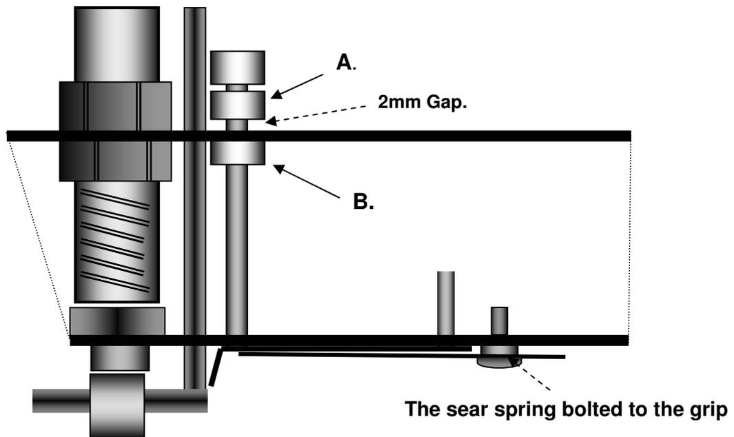
The sear spring consists of a 2-3/8" length of 1/2" x 22 gauge spring steel strip. A 6mm diameter hole is drilled through the spring, 5/8" from one end. In order to attach the spring to the grip, a smaller 5mm hole is drilled 1-3/8" from the grips lower edge. This hole is then tapped to accept a 6mm diameter socket screw.
