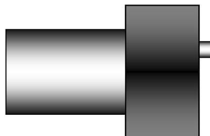
Side view of breech block with firing pin fitted.
