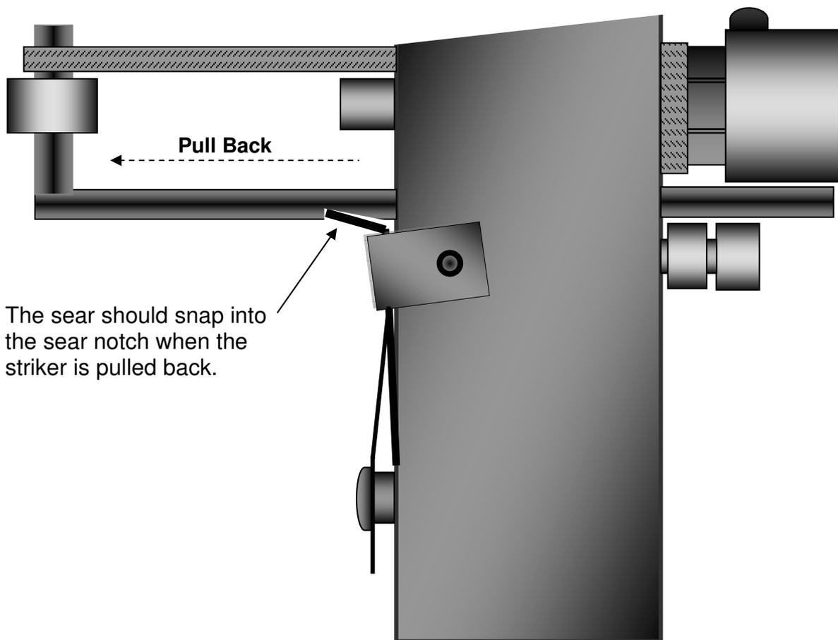
The pistol is shown here in the ready to fire position.
