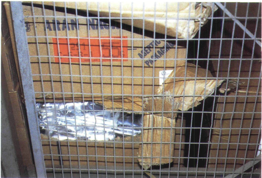
2. The carton on the outer lower conveyor that caused the jam and which the operator worked to free.
