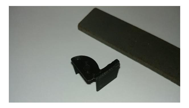
Get the bolt welding jig and sand/file any potentially squished and flat edges so they are rounded.
