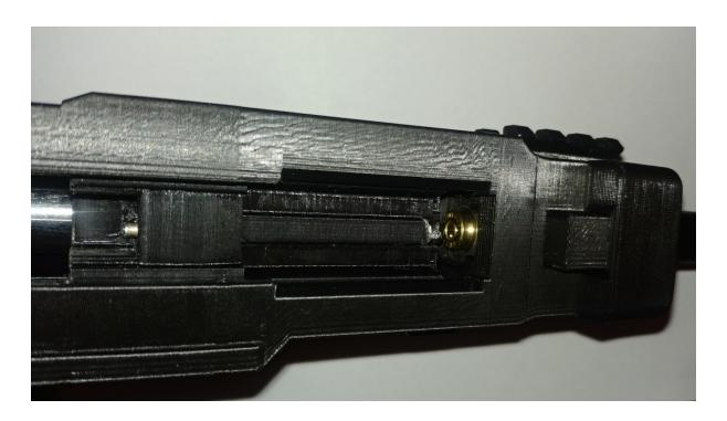
Put the bolt into the bolt carrier without using anything to fix it in place yet, and then put the bolt carrier with the bolt inside into the upper receiver. Turn the upper receiver upside down and look into it from the bottom.
