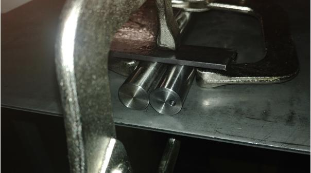
Get your bolt welding jig and a 3.5mm drill bit and use them to make sure that the hole you drilled in the shorter bolt piece is exactly at 3 o'clock.
