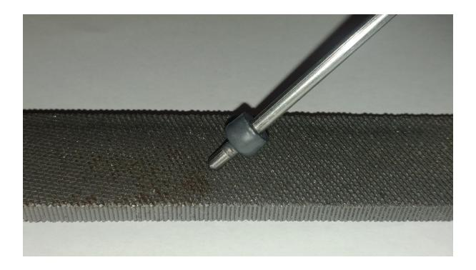
Using a metal file shorten the firing pin by grinding the back end of the firing pin to reach an overall length of 67.50mm.
