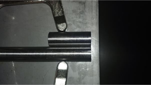
After you have made sure that the drilled hole in the shorter bolt piece is exactly halfway between top and bottom (at the 3 o'clock position) you can remove the bolt jig and the drill bit. Remove the clamp that pressed the bolt pieces against the table and more importantly make absolutely sure that the front ends of the bolt pieces are absolutely flush. Meaning on the front/bolt face the ends should be in line and one bolt should not stick out more than the other.
