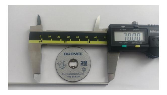
Cut off a 70mm long piece from your 3mm DIA steel bar with a Dremel tool /angle grinder with a steel cutting disc.
