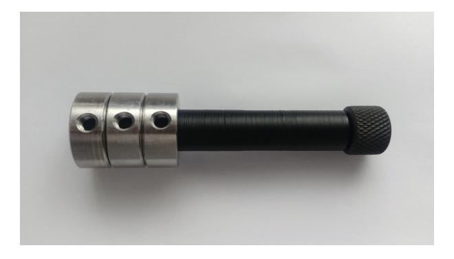
Slide the three shaft collars onto the chamber end of the barrel and have the face of the barrel on the chamber side be flush with the face of the first shaft collar.
