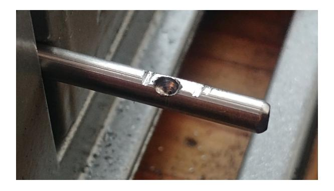
Use your power drill and a 1mm drill bit and then afterwards go deeper with a 2mm drill bit, to create a divot deep in the bar that is in the center of the flat area you created, that is aligned with the previously created line which is 58.35mm from the tip.
