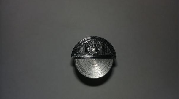
Hold the drilling jig that has the short bolt piece inside and drill into the holes on both sides to mark where you will drill deeper later.
