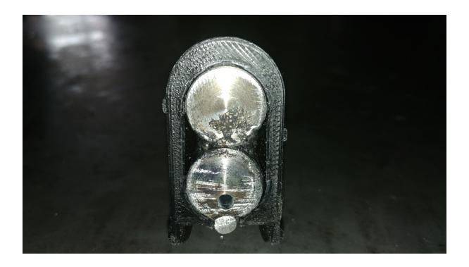
Make sure the bolt sticks out by at least 0.2mm out of the carrier after you are done with all your filing and sanding on the bolt pieces.
