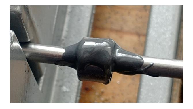
Once you have made sure the shaft collar screw hole is lined up with the divot you previously created by probing with a toothpick, you can fill the hole with JB weld.
