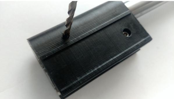
Now put your 4.2mm drill bit in the power drill and try to enlarge that marked spot through the charging handle slot while making sure that the enlarged spot is again between the top and bottom of the charging handle slot. You can now remove the bolt carrier from the upper and drill into the marked spot you created, trying to stay as straight as possible while you drill into the bolt. Make sure you do not cant the drill bit in any way.
