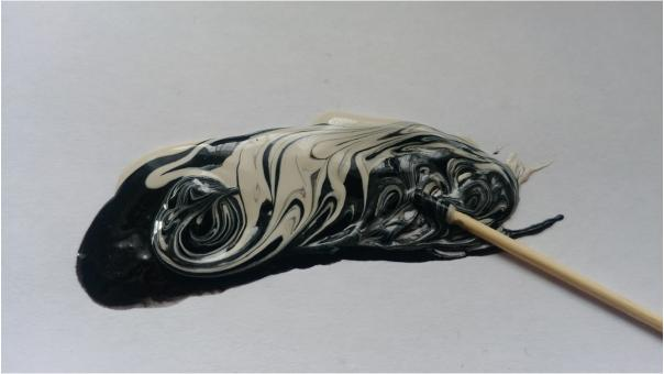
Squeeze an equal amount of both parts of the JB weld compound. Use the toothpick to mix the two parts of the JB weld compound well. After having mixed the JB weld well put it on your toothpick to pick up some JB weld.
