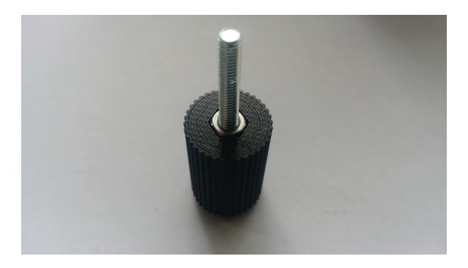
Rotate the nut on the screw in such a way that when you drop it into the charging handle cavity, the outward side of the nut is flush with the flat side of the charging handle.
