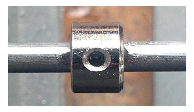
Remove the grub screw from the shaft collar and put the shaft collar onto the bar aligning the hole of it with the divot to get an idea where the shaft collar should be for the later steps.
