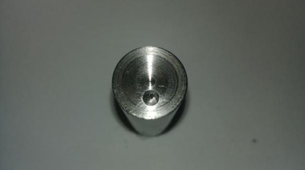
After having both divots/shallow holes on both sides to 3.5mm in diameter get cutting fluid and spray some on the drill bit as well as the hole when drilling deeper.
