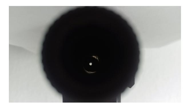
You can look into the muzzle end of the barrel and have the bolt be close to the chamber to make out if the firing pin channel hole is centered with the center of the barrel. In this picture for example the firing pin channel is not centered with the barrel.
