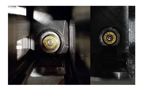
On the left you can see how the indent on the primer is off-center and basically at the 12'o clock position. This is NOT how it should be.
