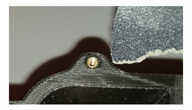
Take sand paper and sand away the uneven surface that was formed by the plastic melting. Make sure to get the surface around the thread insert hole smooth so that the entire back surface is flush.
