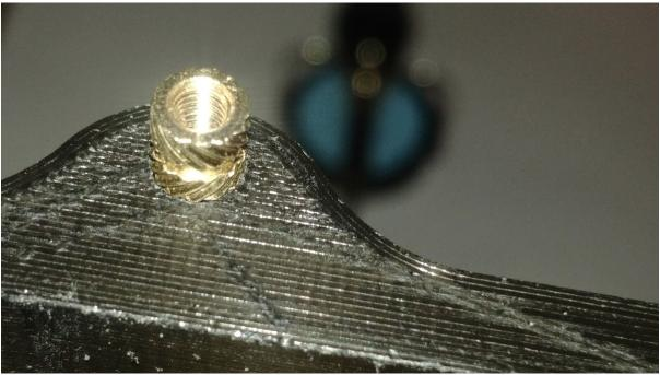
Prepare all four thread inserts as well as the upper receiver and lower receiver. Get your soldering iron and pre-heat it. Put the thread inserts with the tapered side into the holes on the back side of the upper and lower receiver.
