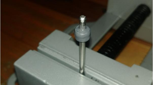
Clean the flat side of the shaft collar that is towards the tip from any JB weld. After you have applied JB weld and cleaned it from the places that should be free of JB weld, as you can see in the picture, let the firing pin cure in a vertical position for at least 24 hours.
