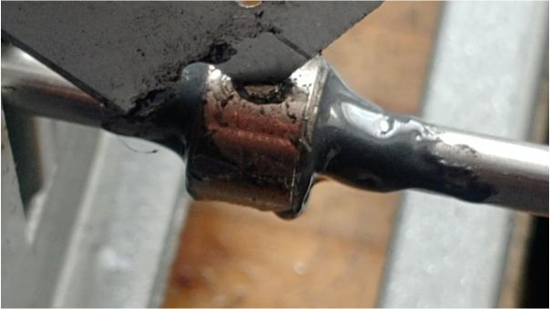
Take a razor blade and apply a drop of grease along the shorter edge of the razor blade to have the grub screw stick to it. Screw the grub screw into the JB Weld-filled shaft collar screw hole. Cover the entire shaft collar and the area behind the shaft collar with JB Weld.
