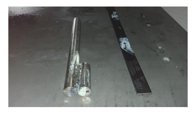
Turn on your arc welder and then set the appropriate amperage which you can find on the packaging of the electrode you will be using, for example when using some 2.5mm diameter electrodes you will need to set your arc welder between 65 and 80 amps.
