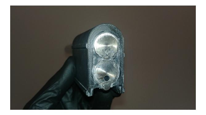
Fill up any gaps and crevices on the bolt face side that is between the inside of the carrier and the bolt, as you can see in the picture and then put the bolt somewhere so that the JB Weld can cure for 24 hours. Make sure that you use something that is appropriate to prop up the longer bolt piece that is sticking out of the bolt carrier to prevent the longer bolt piece from being canted.
