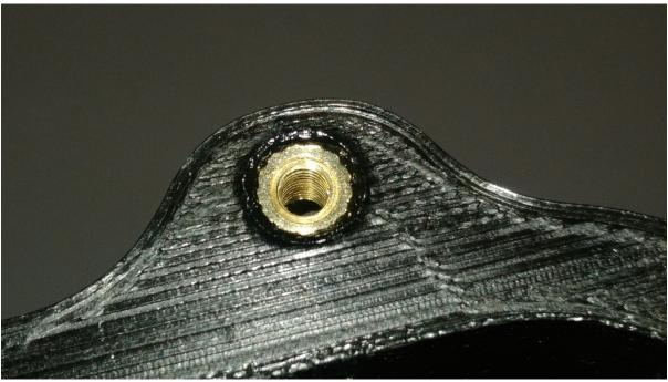
Making sure the thread inserts can go down in straight use your soldering iron to push in the thread inserts about 1-2mm past the entrance of the hole. Meaning the thread inserts should not stick out of the hole.
