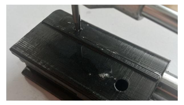
Take your M5 thread tap and secure it into your tap holder properly and start to cut the threads into the hole you just drilled.
