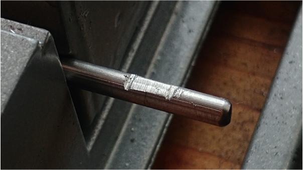
Put the bar into a vise and use the edge of your metal file to create a flat section around the previously marked position.
