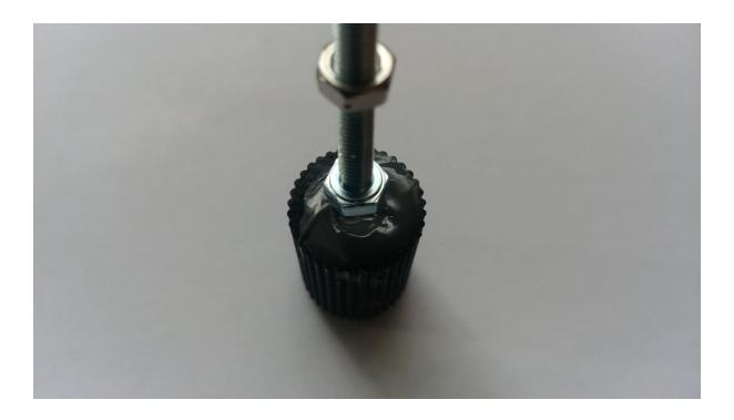
Put the screw with the still attached nut from the state it was in after Step 2, into the charging handle cavity.
