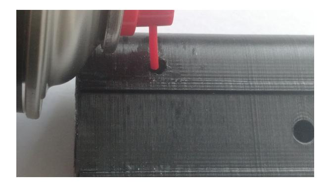
Get cutting fluid into the hole as you start to reach the steel bolt piece inside the carrier while drilling.
