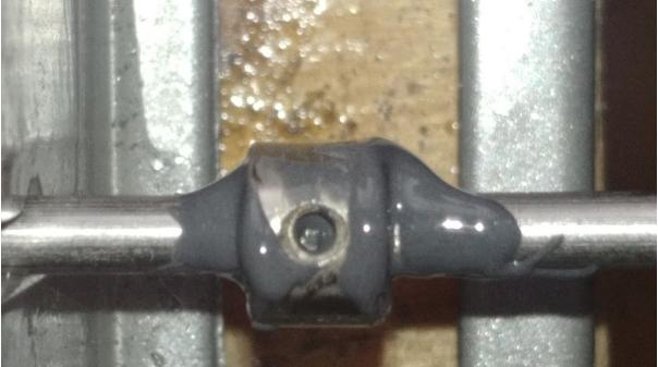
Remove the shaft collar and put some JB Weld onto the flat area that you filed and fill up the drilled divot. Then slide the shaft collar to that position and try to line up the hole with a tooth pick through the hole of the shaft collar.
