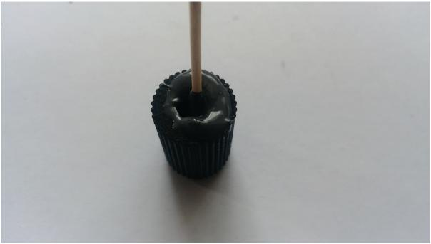
Apply a decent amount of JB weld into the charging handle cavity. Make sure that enough JB weld is in the cavity so that excess JB weld will be pushed out when inserting the screw.
