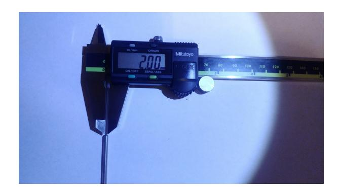
Put the bar into a power drill and rotate it while holding a metal file against it to form a chamfered circle end at the tip that is 2mm in diameter.
