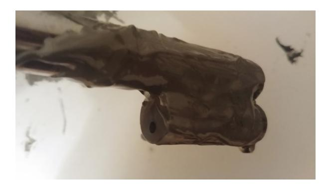
After you have been able to properly file the bolt pick-up into shape and at the same time have the firing pin leave indents into the primer of the cartridge case perfectly in the center you can start mixing up JB weld and applying it as you can see in the photo.
