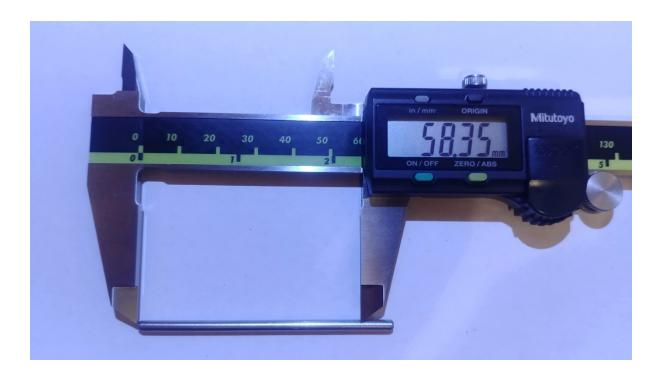
Use your caliper blades to scratch a line around the circumference of the bar at a distance of 58.35mm from the tip.
