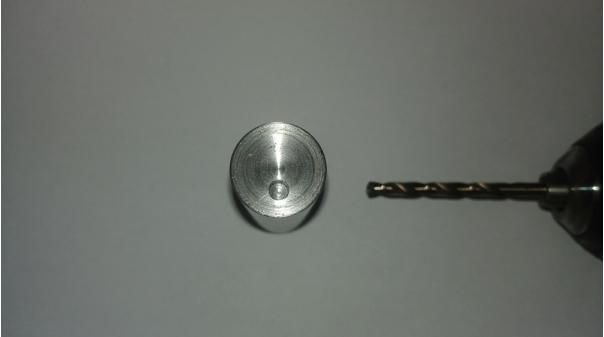
Remove the short bolt piece out of the drilling jig.
