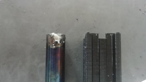
After letting the probably very hot bolt cool off, hold the bolt like in the image while having the bolt always having contact with the metal plate and then put blobs of welding material on the underside near the bolt face of the shorter bolt piece.
