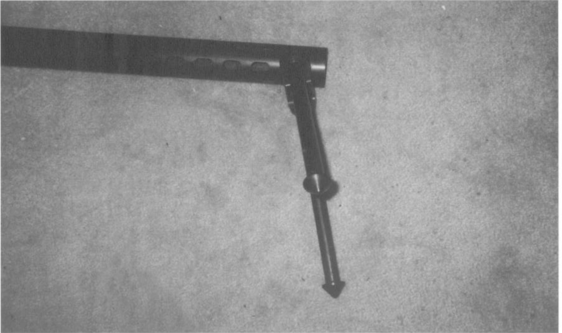
Bipod mounted in place.
