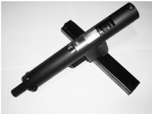
Top: The lack of any external cocking handle further amplifies concealability while it's large port opening ensures reliable ejection.
